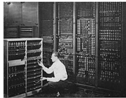
Replacing a bad tube meant checking among ENIAC's 39,000 possibilities.
